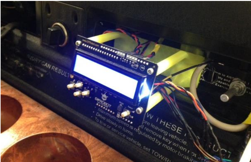
Figure 3. New LCD with 3D-printed mount
